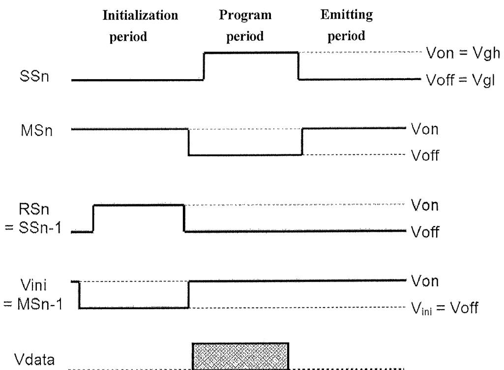
during the initialization period, the first and second reset transistors are turned on to initialize the first and third nodes to the initialization voltage, and a third reset transistor initializes the second node to the high potential voltage in response to the reset signal,
